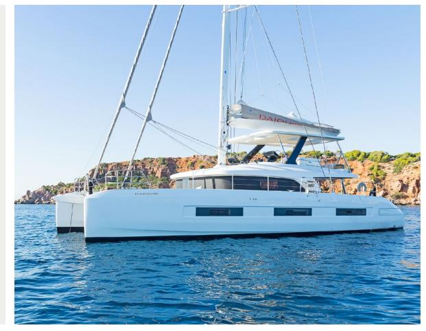
Builder/Type:<br/>Built:Lagoon Sixty 5<br/>2022L.O.A:20,55m 67,50ft<br/>10,00m 32,10ftBeam:<br/>Draft:10,00m 32,10ft<br/>1,55m 5,10ftMain Engines:<br/>Generator:2x 195hp Yanmar<br/>19Kw OnanCruising Speed:<br/>Fuel Consumption:10knots<br/>50lt/hr
